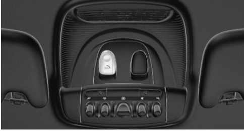
SOS button in the roofliner
